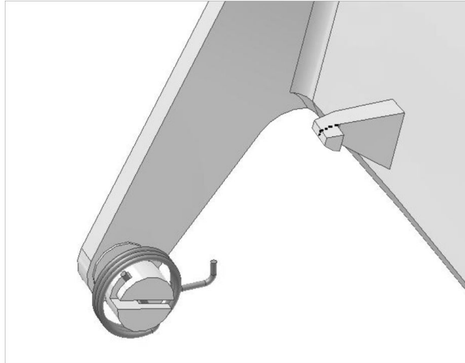
Fig. 9 Cover spring assembly
